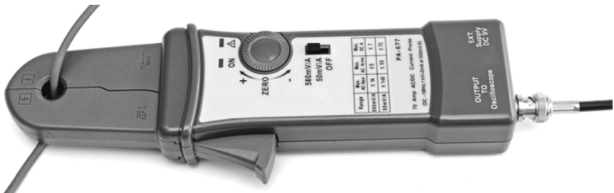
Figure 2: Connecting the PA-677 current probe.
